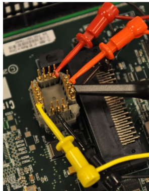
Figure 4-7: EEPROM PLCC32 Testclip on the NVRAM of CISCO1712
