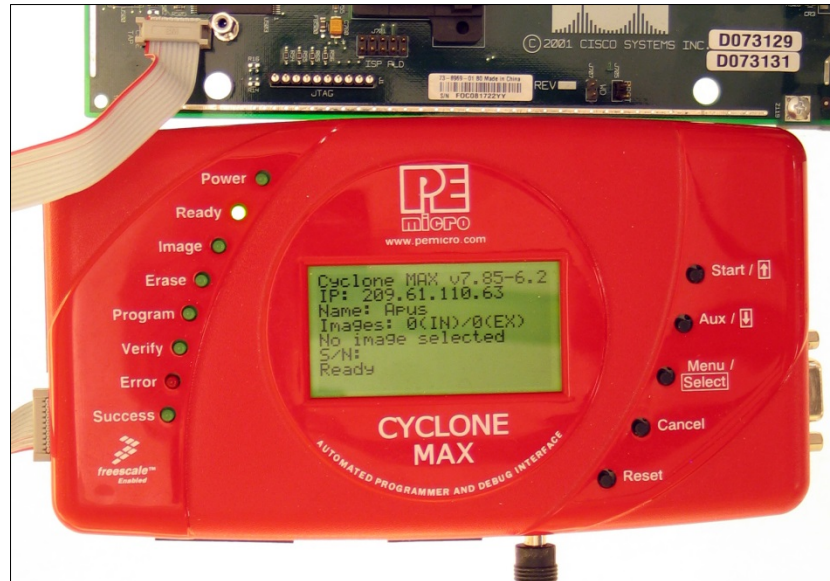
Figure 4-10: Cyclone MAX BDM debugger connected to a CISCO1712 BDM port
